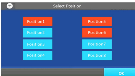
Figure 7: Select Position interface of the CleanXtract 96 with heated positions indicated in red.
