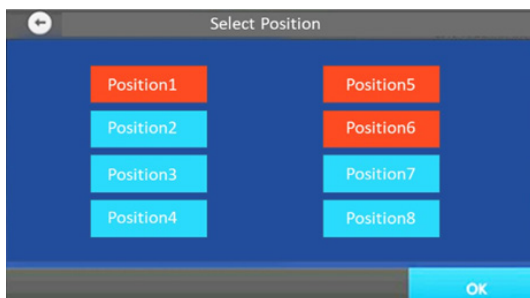
Figure 3: Select Position interface of the CleanXtract 96 with heated positions indicated in red.
