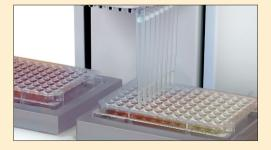
Performing serial dilutions and mixing of entire plates is easily accomplished. The number of mixing cycles and mixing speed can be exactly defined.
