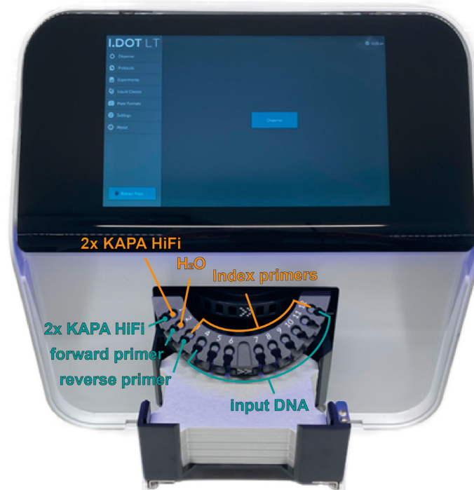
Figure 4: The I.DOT LT non-contact low volume dispenser. Source wells for the amplicon PCR setup are indicated in cyan, and source wells for the indexing PCR set-up are indicated in orange.
