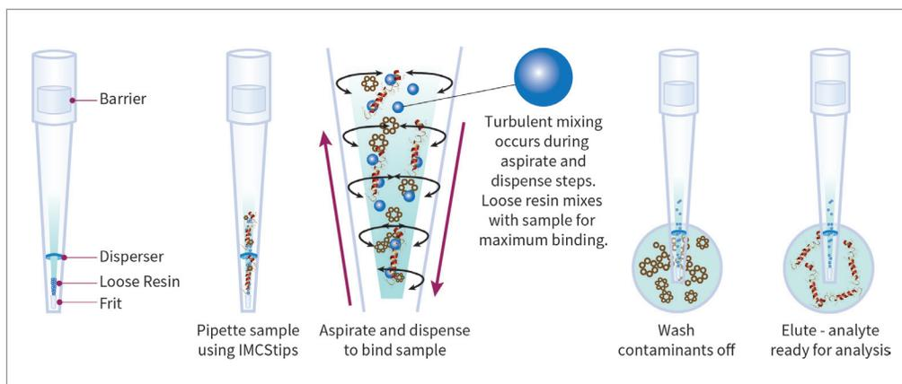
**Figure 1.** IMCStips use a patented dispersive solid-phase extraction (dSPE) technology. Unlike fixed-bed SPE (fbSPE) devices, IMCStips contain loosely packed resins that mix with sample solutions during aspirate and dispense cycles (mixing cycles), ensuring maximum contact between the resin and analytes of interest. Turbulent mixing within the tip is further enhanced by the addition of a patented disperser. Purification follows a typical bind, wash, elute workflow.
