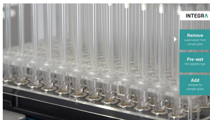
Figure 5: Separating the magnetic beads from the PCR samples.
