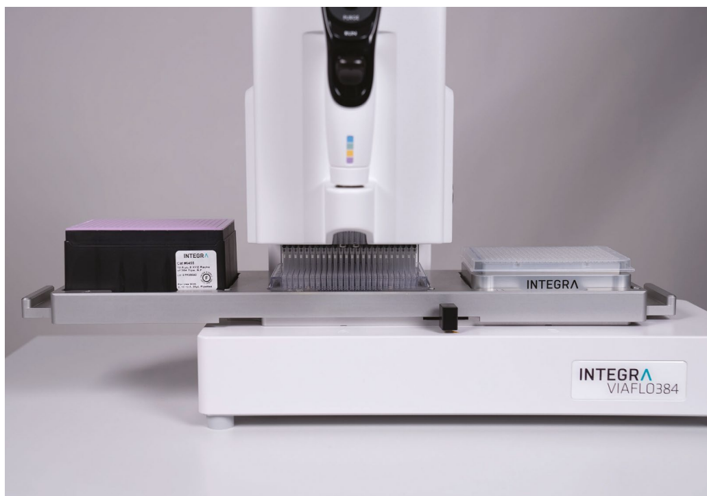
Figure 3: The three position stage of the VIAFLO 384 set up for the cell lysate transfer step.
