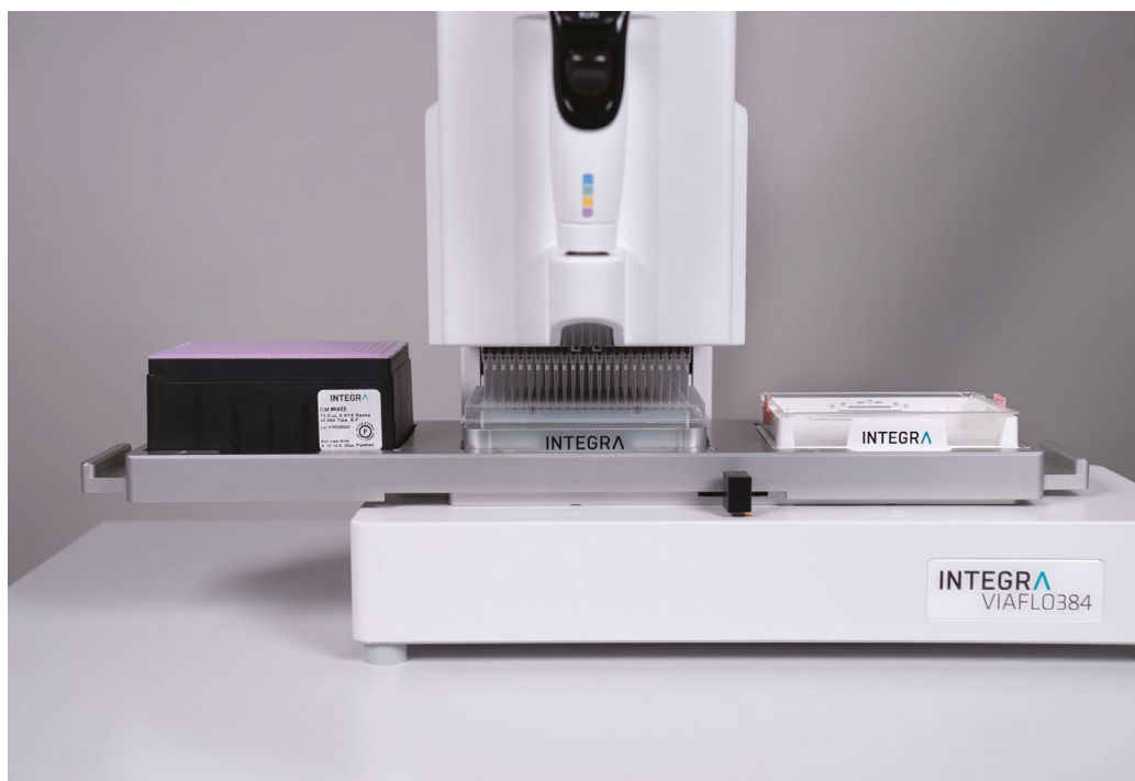
Figure 5: The three position stage of the VIAFLO 384 set-up for the pooling step.
