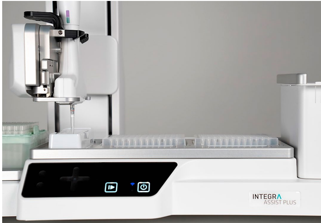
Figure 5: The D-ONE single channel pipetting module transfers the required volume of diluent to each well.
