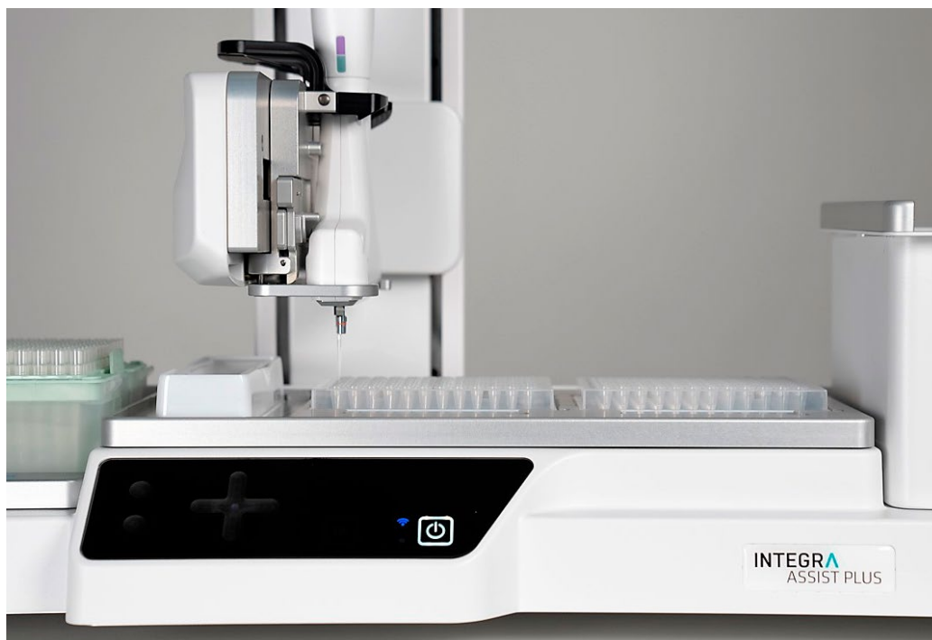
Figure 6: The D-ONE single channel pipetting module transfers the samples individually.
