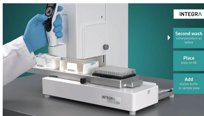
Figure 7: Elute samples from the magnetic beads.
