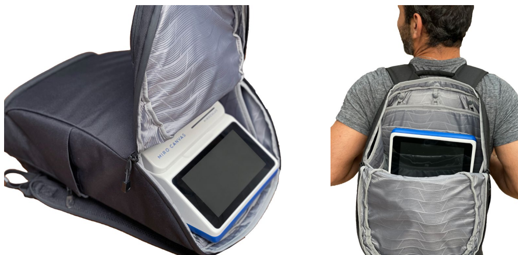
Figure 5: The MIRO CANVAS's compact dimensions (20.2 cm W x 40.6 cm D x 17.6 cm H) make it easy to packed for travel, providing the ideal companion for ONT's portable sequencers.
