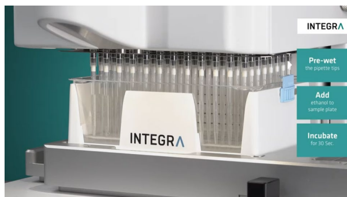
Figure 6: Wash the magnetic beads twice with 70 % ethanol.
