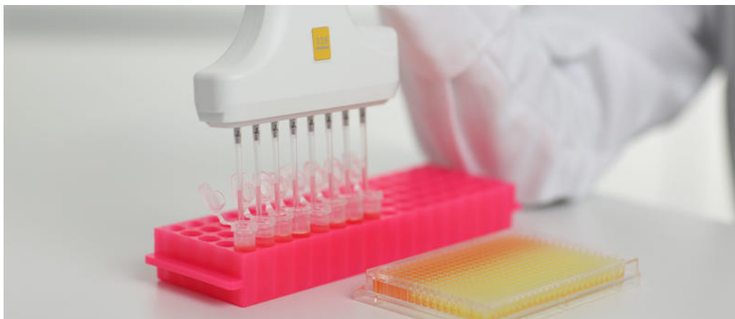
Figure 2: VOYAGER is the only automatic adjustable tip spacing pipette on the market.
