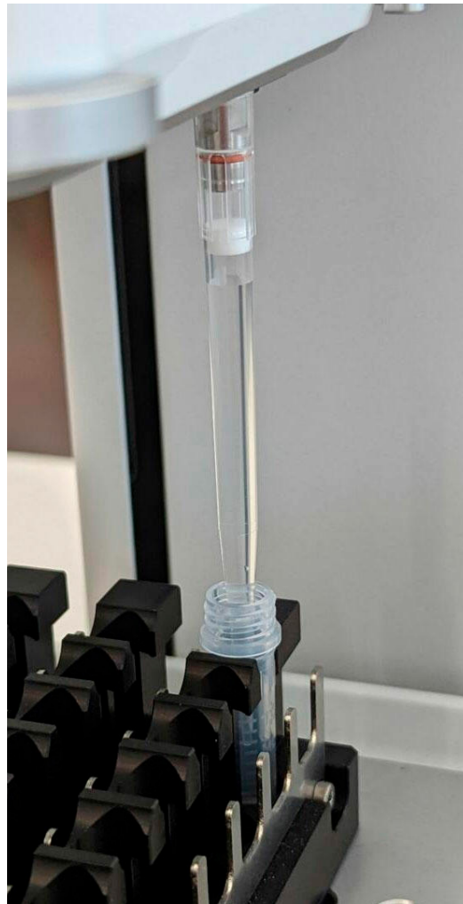
Figure 8: Reagent aliquoting from a manufacturer tube with the D-ONE pipetting module.
