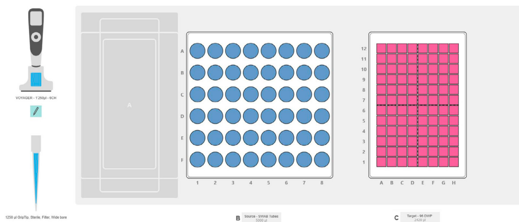
Figure 2: Deck set-up for sample transfer from swab tubes to 96 deep well plate. Position A: Empty. Position B: INTEGRA rack for swab tubes (blue). Position C: 96 deep well plate (magenta).
