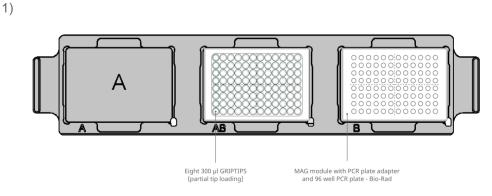
After partial tip loading, the pipette will prompt you to slide the stage to the left and to load the deepwell plate containing the magnetic beads onto position A/B.
