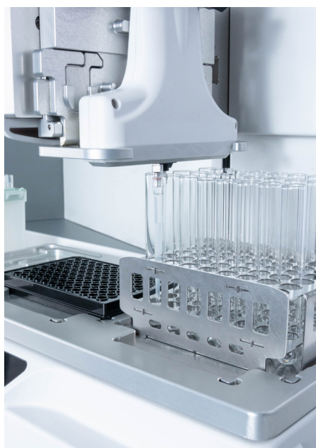
Figure 3: LAL water is dispensed by the D-ONE single channel pipetting module.
